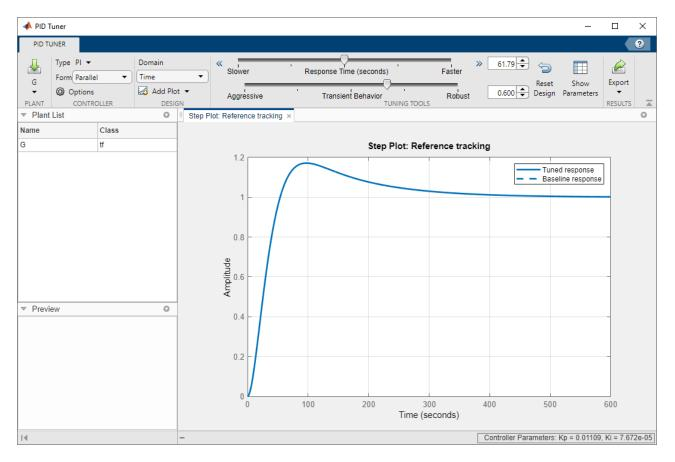
Add a step response plot of the input disturbance rejection. Select **Add Plot > Input Disturbance Rejection**.
