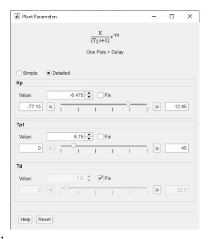
Automatically optimize the system parameters to match the measured response data. Click **Auto Estimate** to update the estimated system parameters using the current values as an initial guess.
