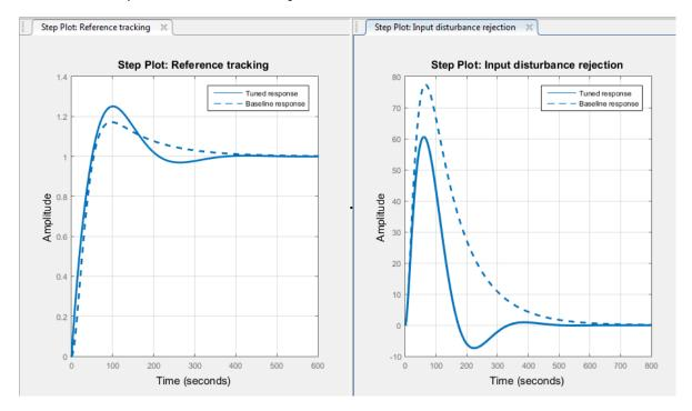
This controller design yields improved disturbance rejection, but results in some increased overshoot in the reference-tracking response.
