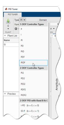
**PID Tuner** automatically designs a controller of the new type, PIDF. Move the **Transient Behavior** slider to set the coefficient back to 0.6.
