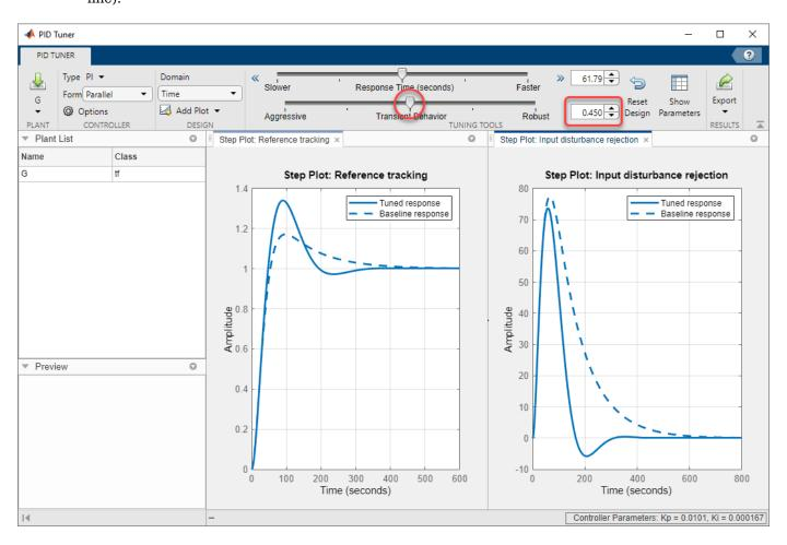
Lowering the transient-behavior coefficient to 0.45 speeds up disturbance rejection, but also increases overshoot in the reference-tracking response.
