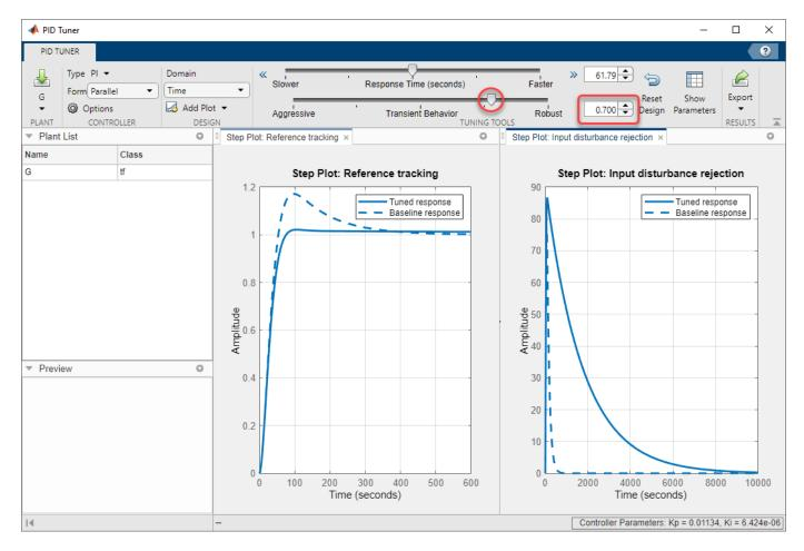
Increasing the transient-behavior coefficient to 0.70 nearly eliminates the overshoot, but results in extremely sluggish disturbance rejection. You can try moving the **Transient behavior** slider until you find a balance between reference tracking and disturbance rejection that is suitable for your application. The effect that changing the slider has on the balance depends on the plant model. For some plant models, the effect is not as large as shown in this example.
