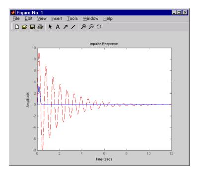
**Comparison of Open- and Closed-Loop Impulse Response**
