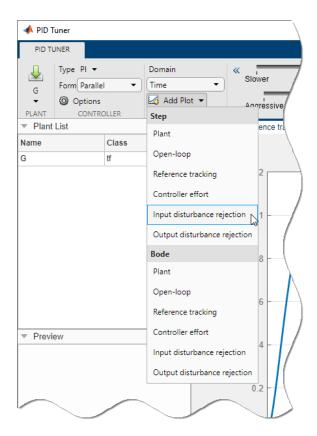
PID Tuner tiles the disturbance-rejection plot side by side with the reference-tracking plot.
