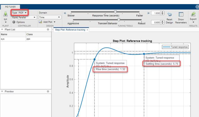
In the **Type** menu, select PIDF. **PID Tuner** designs a new PIDF controller. (See "PID Controller Type" on page 4-5 for more information about available controller types.)
