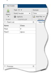
You can now use the **PID Tuner** tools to refine the controller design for the estimated plant and examine tuned system responses.
