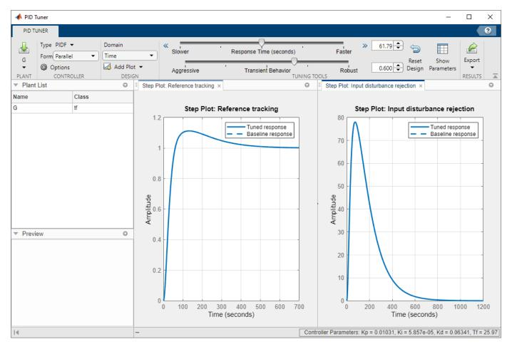
Change the **PID Tuner** design focus to favor reference tracking without changing the response time or the transient-behavior coefficient. To do so, click **Options**, and in the **Focus** menu, select Reference tracking.
