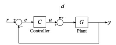
Setpoint tracking is the response at y to signals at r. Input disturbance rejection is the suppression at y of signals at d.
