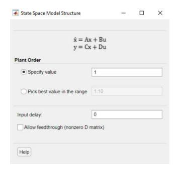
Use the dialog box to specify model order, delay and feedthrough characteristics. If you are unsure about the order, select **Pick best value in the range**, and enter a range of orders. In this case, when you click **Estimate** in the **Plant Estimation** tab, the software displays a bar chart of Hankel singular values. Choose a model order equal to the number of Hankel singular values that make significant contributions to the system dynamics.
