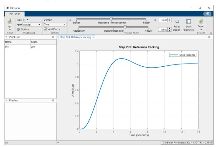
When you open **PID Tuner**, it automatically designs a controller of the type you specify (here, PI). The controller is designed for a balance between performance (response time) and robustness (stability margins). **PID Tuner** displays the closed-loop step response of the system with the designed controller.
