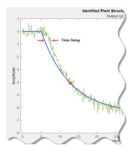
To add a transport delay to the estimated plant model, in the **Plant Structure** section, check **Delay**. A vertical line appears on the plot, indicating the current value of the delay. Drag the line left or right to change the delay, and make further adjustments to the system response by dragging the red x.
