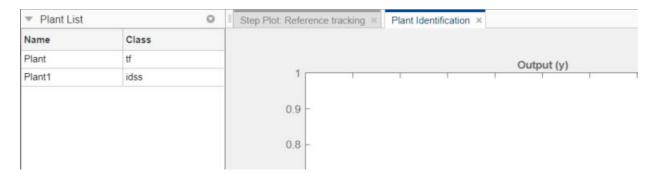
You can define the model structure and initialize the model parameter values using one of these plants. To do so, in the **Plant Identification** tab, in the **Structure** menu, select the linear plant model you want to use for structure an initialization.
