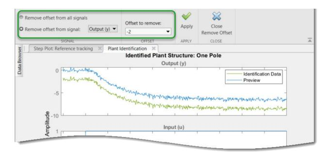
Click Apply to save the change to the signal. Click Close Remove Offset to return to the Plant Identification tab.
